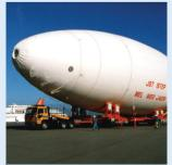
Airship constructed with VECTRAN
